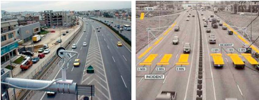
**Figure 1.3** Video image processing system. (Photos from <http://www.imagesensing.com/>)
