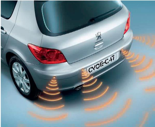
**Figure 1.6** Acoustic/ultrasonic sensors. (Photo from <http://autoteksheffield.co.uk/security/parking-sensors/>.)
