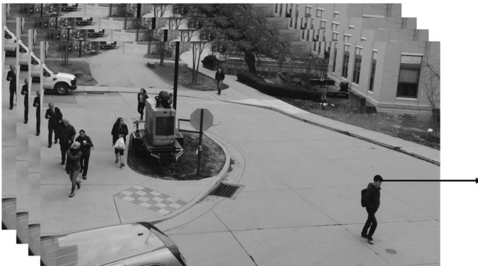
Figure 10.3 Pixels of a video sequence processed for background/foreground detection, capturing changes occurring due to the passing man.
