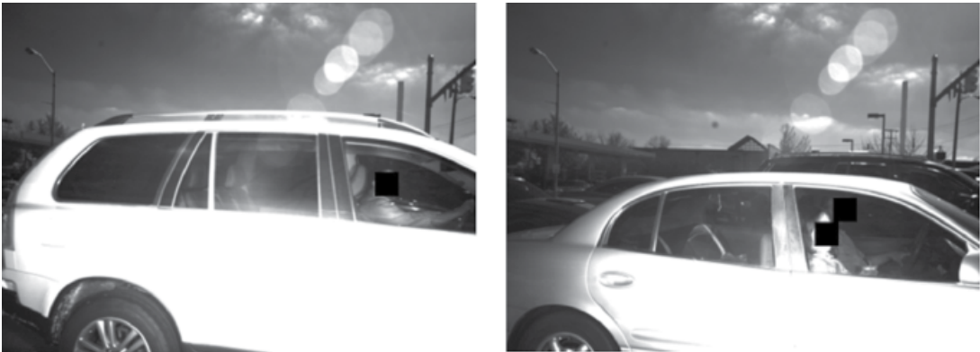
Figure 4.2 NIR images acquired by HOV/HOT lane front- and side-view cameras: (a) front-view images and (b) side-view images.
