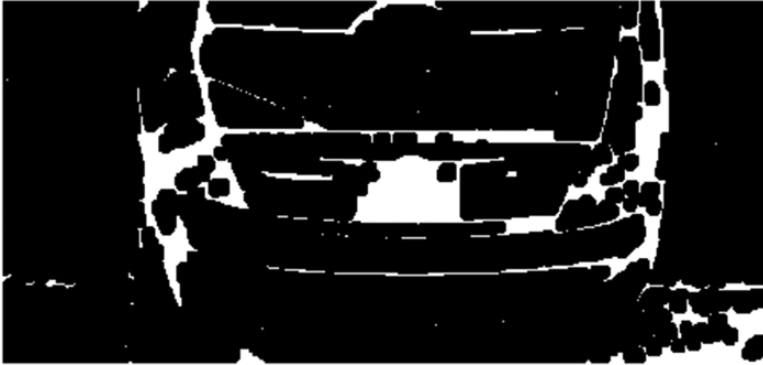
Figure 2.4 Results of morphological close operation on edge image.
