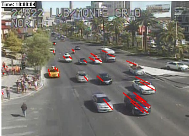
Figure 7.4 Tracking features of two frames using the KLT algorithm.
