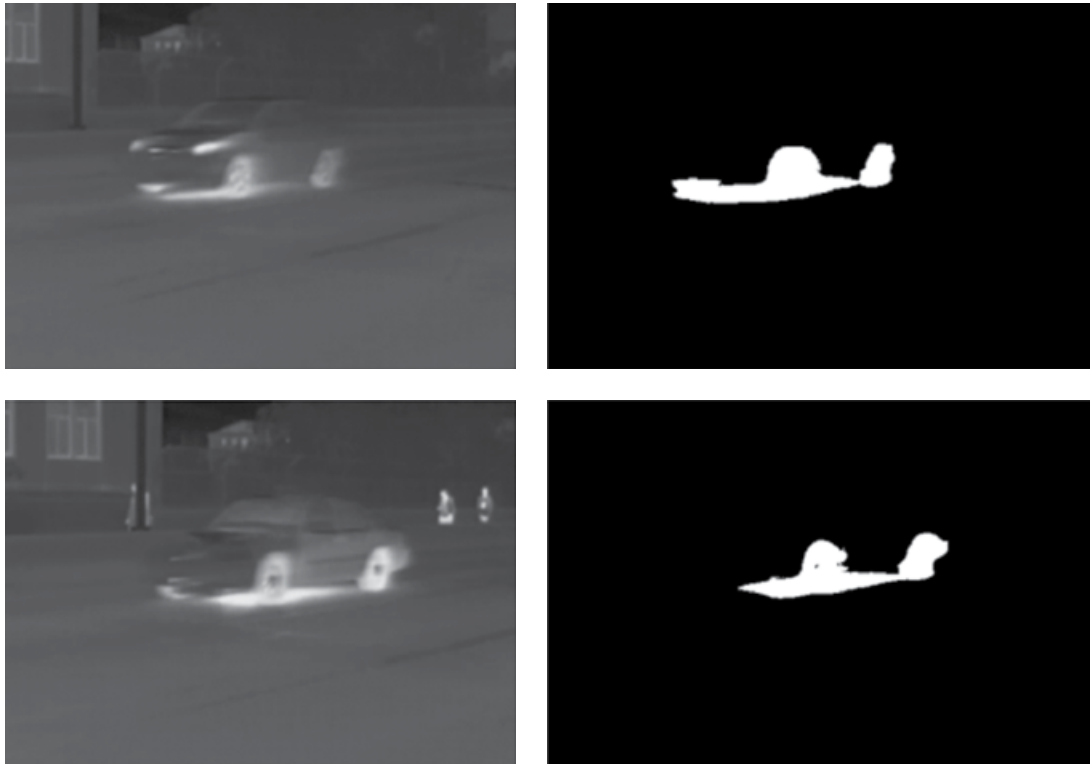
Figure 3.10 Heat signature extracted from image of a car.
