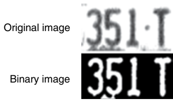
Figure 2.19 Difficult example for projective segmentation.
